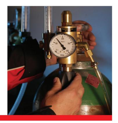
ARGON/CO<sub>2</sub> REGULATOR WITH FLOW METER AND INTEGRATED GAS SAVER FUNCTION
