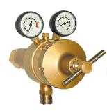
"S1510L2" SERIES – this pipeline regulator is ideal for tank systems, rear entry to suit panel or line mounting. The larger outlet configuration is necessary to give high flow from a relatively low inlet pressure source. Max inlet 24 bar and delivery up to 10 bar.
