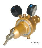
"OR14" SERIES – offering some of the highest flows in the GCE BUTBRO range through the use of a special monel tied valve, these are intended for cylinder and pipeline applications. The G5/8 inlet adaptor can be removed to reveal a1" BSP flat seat female fitting. Range up to 14 bar delivery pressure.
