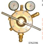
"M600" SERIES – improved delivery pressure control is achieved from two stage regulation. Typical applications are those left unattended for periods of time such as cable pressurisation, chemical and laboratory. Range up to 41 bar delivery pressure.
