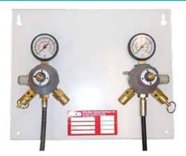
Basic one cylinder panel for both  ${\rm CO_2}$  and mixed gas, suitable for connection into a blender system, (can be connected to kegs only if additional secondary regulators are used downstream).
