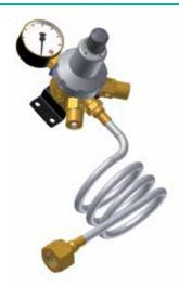
This wall-mounted twin regulator for  $CO_2$  is fitted in the higher pressure of a soft drinks single ring main. To used in conjunction with single wall mounted  $CO_2$  primary regulator or bulk supply from other source. Standard outlet fittings are 3/8" John Guest.
