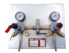
This wall-mounted panel connects two or more  $\mathrm{CO}_2$  cylinders to a single ring main, kegs, or soft drinks systems, depending on the delivery pressure/relief valve selection. Two single stage regulators and a low pressure changeover valve are mounted on a panel, with standard outlet fitting 3/8" John Guest. Please specify system application to ensure correct safety valves are employed.
