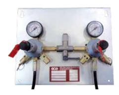
This wall-mounted panel connects two or more Mixed Gas cylinders to a single ring main, kegs, or soft drinks systems, depending on the delivery pressure/relief valve selection. Two single stage regulators and a low pressure changeover valve are mounted on a panel, with standard outlet fitting 3/8" John Guest.
