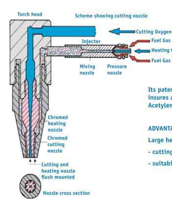
Its patented safety injector design (double safety-injector) insures a maximum of flashback safety independant of the Acetylene pressure level.
