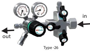
**Single-stage, with inert gas purging, for reactive, flammable, oxidizing and corrosive gases and gas mixtures, not for oxygen, purity max. 6.0, cylinder pressure 230 bar downstream pressure range 0.5 - 200 bar /7 - 2900 psi**
