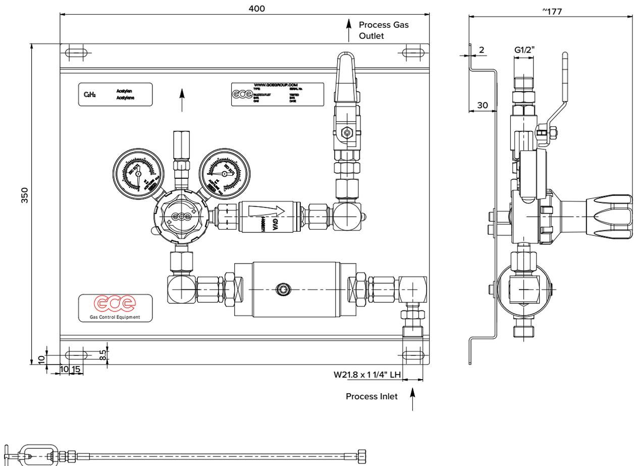
Inlet pressure hose according to the relevant national standard including the check valve
